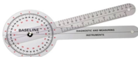
Fig. 1s. The goniometer was used to assess the angle of shoulder flexion, extension, abduction, adduction, elbow and wrist flexion and extension, forearm pronation-supination and flexion of the metacarpal-phalanx joint of the index.
