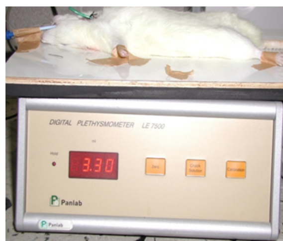
Fig. 3. Example of GV displayed by the plethysmometer (note the close proximity of the experimental rat model)
