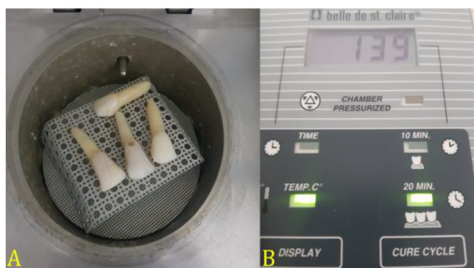
Image 1. Dental sample dehydration (A) in thermobaropolymerization oven; dehydration parameters (B)
